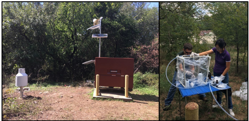
Left: A “super gage” measures surface and groundwater levels and collects rainfall, water quality, and stormwater runoff samples from adjacent streams using an autosampler (that is triggered by water levels indicating stormwater flow). Right: Members of the UHN team collect and process water-quality samples. Photos: USGS
